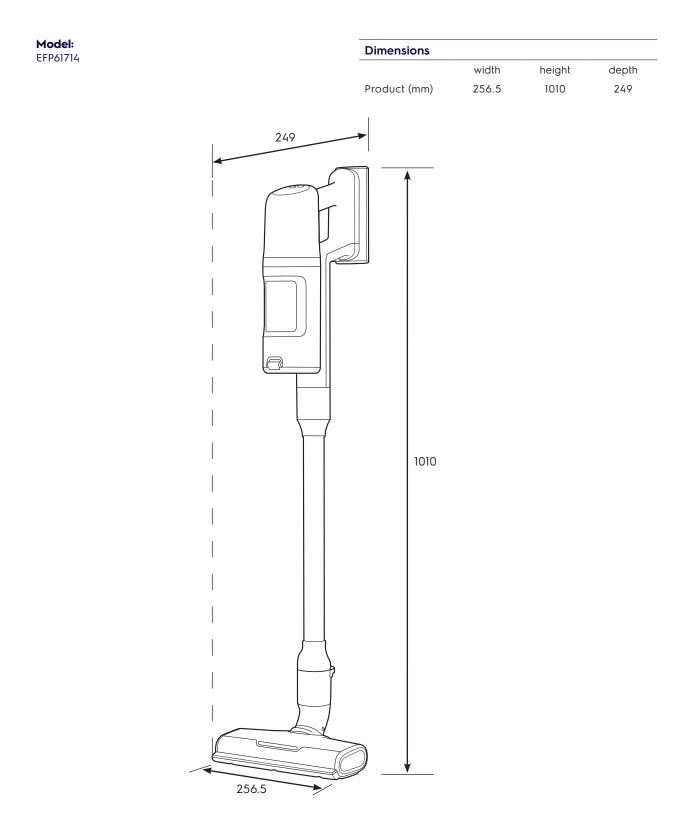
Please note! Dimensions to be used as a guide only. All customers MUST refer to the user manual supplied with the product for detailed installation instructions. © 2024 Electrolux S.E.A PTE. LTD. ELX\_DIM\_EFP61714\_Sep24
