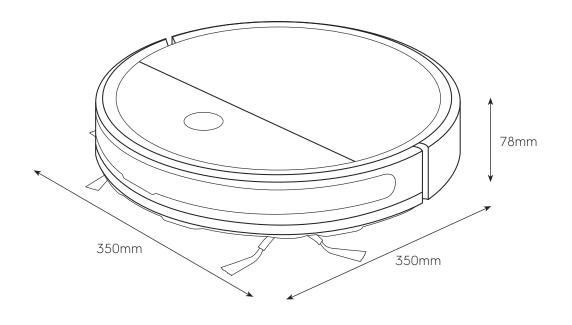
Please note! Dimensions to be used as a guide only. All customers MUST refer to the user manual supplied with the product for detailed installation instructions. © 2021 Electrolux S.E.A PTE. LTD. E\_DIM\_EFR31223\_Jun22
